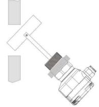
2.The sickle shape paddle can be mounted on the container directly: Insert the paddle to the G1-1/2 inches hole by curving path and tight it on the container.
